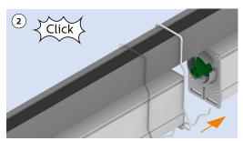
**2)** Hook the next bracket (**A**) onto the C-profile at 1.25 m distance. Put the 2nd module against the C-profile. Slide the 2nd module over bracket (**A**). Connect both modules, verify that these 2 modules are snapped together correctly (click) and check if bracket (**A**) snaps into both end caps of the modules.
