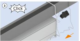
3) Repeat step 2 until the maximum permissible number of modules is reached. For the maximum number of modules allowed per phase, see page 10. Slide the 4th bracket (A) into the last module. IMPORTANT: Put the plastic end cap into the female connector (click) of every last module, to comply to IP66, no dewing allowed.
