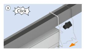
**3)** Repeat step 2 until the maximum permissible number of modules is reached. For the maximum number of modules allowed per phase, see page 10. Slide mounting bracket (**A**) into the last module. **IMPORTANT:** Put the plastic end cap at the end of a through wire line (click) to comply to IP66, no dewing allowed.
